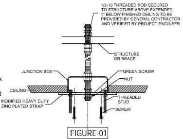
2. Fasten the ground wire to the green or bare copper wire in the outlet box of the green screw on the mounting strap.
