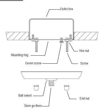
5. Fasten the white fixture lead to white wire in the outlet box.
