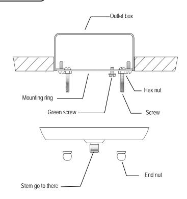
5. Fasten the white fixture lead wire to the white wire in the outlet box. Fasten the wires together with an approved fastener (wire nut). Starting about 1" below the fastener, Tightly wrap the connection with electrical tape so that the connection seals the end of the fastener.
