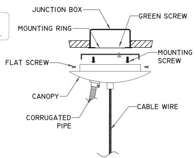
3. Fasten the white fixture lead to the white wire in the junction box. Fasten the wires together with an approved fastener (wire nut). Starting about 1" below the fastener, tightly wrap the connection with electrical tape so that the connections seals the end of the fastener.
