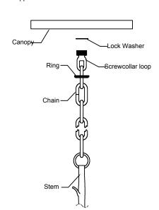
3. Open the end links of the chain and attach the chain to the screw collar loop. hang the fixture on the chain at the desired height. Remove the excess chain close all links. Unscrew the threaded ring from the screw collar loop. Allow the ring and canopy to side down the chain to the top of the fixture.
