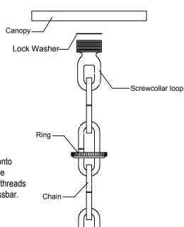
3. Open the end links of the chain and attach the chain to the screw collar loop. hang the fixture on the chain at the desired height. Remove the excess chain close all links. Unscrew the threaded ring from the screw collar loop. Allow the ring and canopy to side down the chain to the top of the fixture.
