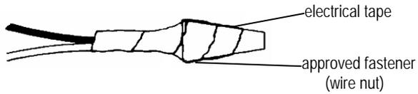
4. Connect the black fixture lead wire to the black wire in the outlet box. Fasten the joined wires as in step 3.
