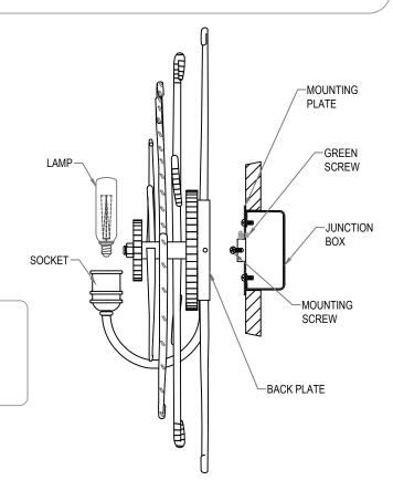
3. Fasten the white fixture lead to the white wire in the junction box. Fasten the wires together with an approved fastener (wire nut). Starting about 1" below the fastener, tightly wrap the connection with electrical tape so that the connections seals the end of the fastener.
