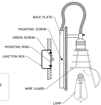
3. Fasten the white fixture lead to the white wire in the junction box. Fasten the wires together with an approved fastener (wire nut). Starting about 1" below the fastener, tightly wrap the connection with electrical tape so that the connections seals the end of the fastener.
