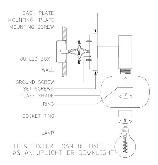
WIRE NUT/TAPING DIAGRAM
