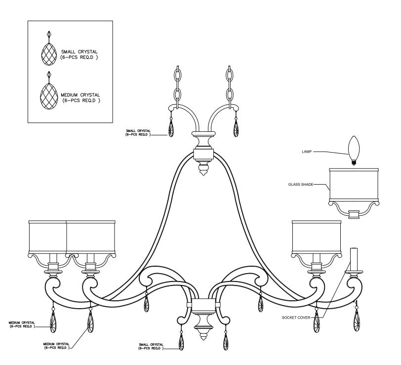
**3.** Open end links of the chains and attach the chains to the canopy loops. Hang the fixture on the chains and adjust to the desired height. Remove excess chain. Close all chain links.
