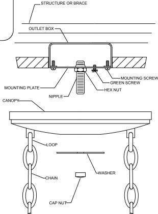
**3.** Open end links of the chains and attach the chains to the canopy loops. Hang the fixture on the chains and adjust to the desired height. Remove excess chain. Close all chain links.
