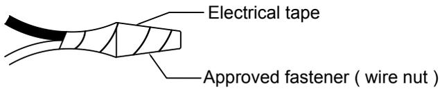
5. Connect the black fixture lead to the black wire in the outlet box. Fasten the joined wires as in step 4.
