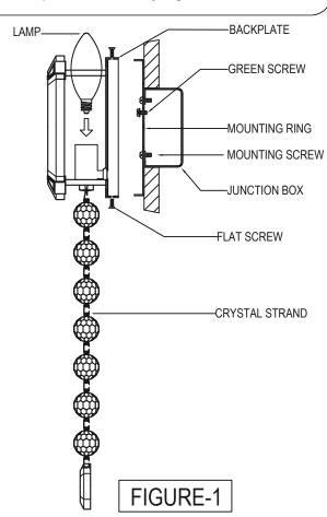
3. Fasten the white fixture lead to the white wire in the junction box. Fasten the wires together with an approved fastener (wire nut). Starting about 1" below the fastener, tightly wrap the connection with electrical tape so that the connections seals the end of the fastener.
