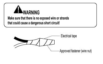
4. Connect the black fixture lead to the black wire in the junction box. Fasten the joined wires as in step 3.
