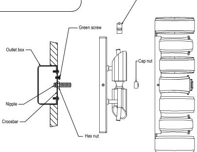
Fasten the ground wire to the green or bare copper wire in the outlet box (if outlet box is plastic) or to the green screw on the crossbar.
