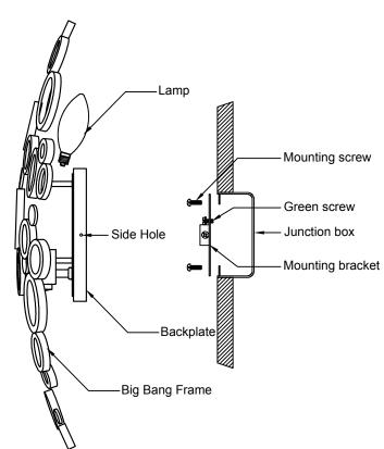
2. Fasten the ground wire to the green or bare copper wire in the junction box or the green screw on the mounting ring.
