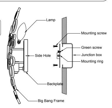
3. Fasten the white fixture lead to the white wire in the junction box. Fasten the wires together with an approved fastener (wire nut). Starting about 1" below the fastener, tightly wrap the connection with electrical tape so that the connections seals the end of the fastener.
