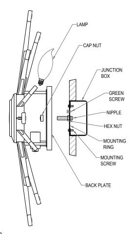
**3.** Fasten the bare ground wire to the green or bare copper wire in the junction box (if junction box is plastic) or to the green screw on the mounting ring.
