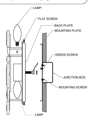
3. Fasten the white fixture lead to the white wire in the junction box. Fasten the wires together with an approved fastener (wire nut). Starting about 1" below the fastener, tightly wrap the connection with electrical tape so that the connections seals the end of the fastener.
