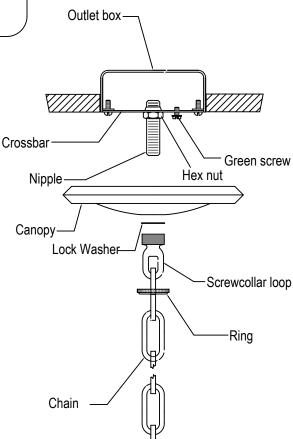
3. Open the end links of the chain and attach the chain to the screwcollar loop. Hang the fixture on the chain at the desired height. Remove the excess chain close all links. Unscrew the threaded ring from the screw collar loop. Allow the ring and canopy to side down the chain to the top of the fixture.
