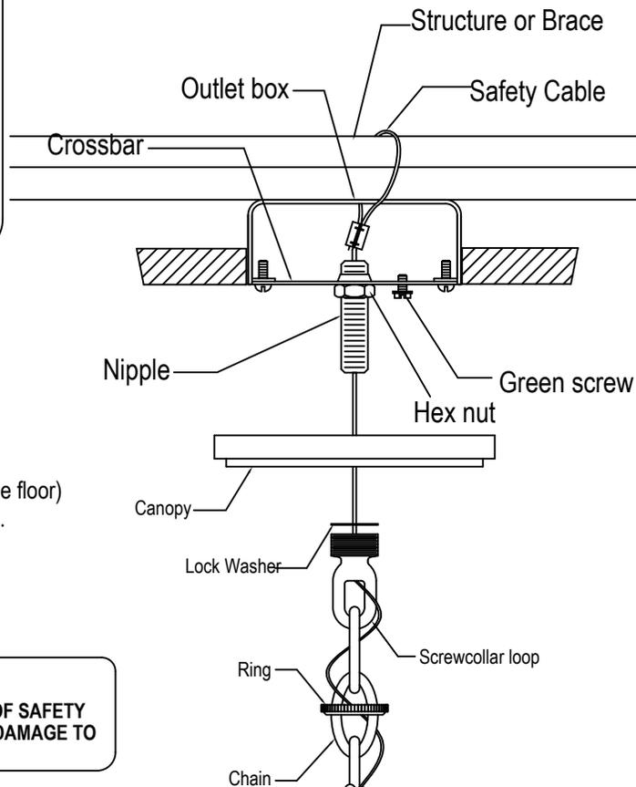
3. Open end links of chain. Attach the chain to the screw collar loop.
