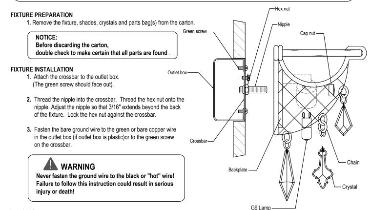
**4.** Fasten the white fixture lead to the white wire in the outlet box. Fasten the wires together with an approved fastener (wire nut). Starting about 1" below the fastener, tightly wrap the connection with electrical tape so that the connections seals the end of the fastener.
