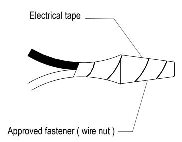
4. Fasten the white fixture lead to the white wire in the outlet box. Fasten the wires together with an approved fastener (wire nut). Starting about 1" below the fastener, tightly wrap the connection with electrical tape so that the connections seals the end of the fastener.
