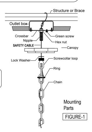
3. Open the end links of the chain. Attach the chain to the screw collar loop. Hang the fixture on the chain at the desired height. Remove excess chain. Close the chain links. Unscrew the ring from the scrwe collar loop. Allow the ring and canopy to slide down the chain to the fixture.
