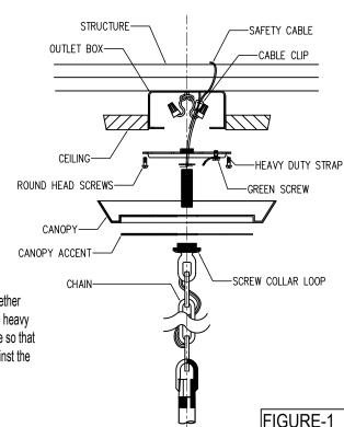
3. Open the end links of the chain and attach the chain to the screw collar loop. Hang the fixture on the chain at the desired height. Remove the excess chain close all links. Unscrew the threaded ring from the screw collar loop. Allow the ring and canopy to slide down the chain to the top of the fixture.
